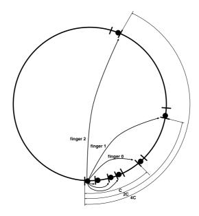
**Fig. 1.** An instance of a chordal ring. Each peer is responsible for a contiguous interval of overlay addresses. Each peer has links to some successors, and other links called "fingers" pointing to peers at distances C, 2\*C, 4\*C, etc., where C is a parameter of the system. With N participants, each peer "knows" O(log(N)) other peers, and can easily infer their overlay addresses thanks to the above geometric progression.
