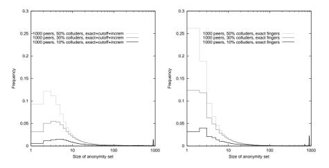
Fig. 7. Average frequency distribution of sender anonymity in simulated chordal rings with 1000 peers and three different percentages of attackers. Left: "hybrid" system with traditional fingers, cutoff distance spanning 10 peers, and incrementally built fingers. Right: traditional Chord system with exact fingers. The differences only affect the regions of very low and very high anonymity.
