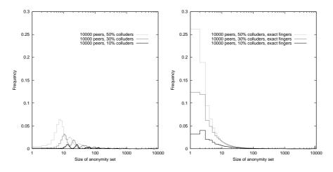
Fig. 6. Average frequency distribution of sender anonymity in simulated chordal rings with 10000 peers and both imprecise and traditional fingers, with three different percentages of attackers. The spikes at right, corresponding to the cases when messages are not intercepted, are too small to be visible. All curves are heavily affected by the x scale being logarithmic; this must be taken into account when comparing curves from different scenarios.
