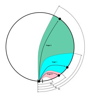
**Fig. 3.** A chordal ring (successors omitted) in which the fingers are affected by an unknown random error. The average error increases proportionally with the distance of the peer. This way, no peer can infer much about the overlay addresses of other peers, and this improves recipient anonymity. Yet, O(log(N)) hops are still sufficient to route messages towards an arbitrary destination.
