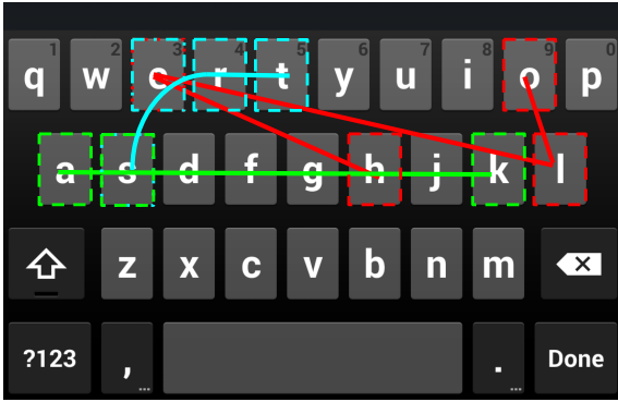
Fig. 1. Path of finger during input of word “hello” (red), “ask” (green) and “très” (light blue).
