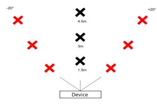
Fig. 3. Experimental setup for the performance evaluation. Participants stood at each X (1.5m, 3m, or 4.5m from the device) and attempted to activate the device. The red Xs are angled 20 degrees from the device, and were only used for gaze evaluation.
