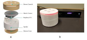
Fig. 1. Our smart speaker prototype: (a) schematic breakdown and (b) prototype with Kinect sensor used for voice-volume-based and gaze-based privacy controls.
