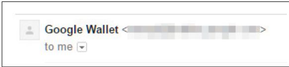
Fig. 10. Example of an email address redacted by mosaicing. Our HMM-based recognizer recovers the text noreply@wallet.google.com , which is the correct address.
