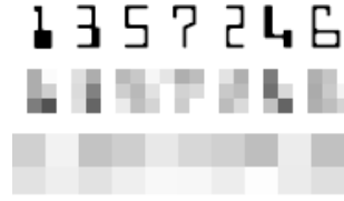
Fig. 5. Top row: a seven-digit string rendered in 24p MICR Encoding font. Middle and bottom rows: mosaiced images with grid sizes of 8p and 18p, respectively.
