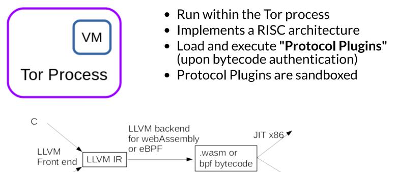
Rust JIT ARM Protocol Plugins, from high-level code to machine code
