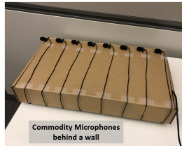
Fig. 2. Adversary microphone array, separated with the user by 6 meters and with a wall in between.
