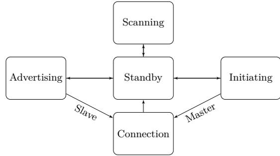
Fig. 1. The Link Layer State machine [20, p. 15].
