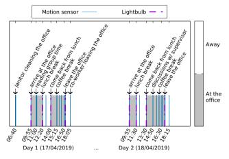
Fig. 17. Representation of the GSN changes extracted from HomeKit messages during two days. For both the motion sensor and lightbulb, GSN changes can be leveraged as an indicator of the presence and activity of a user.
