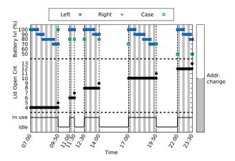
**Fig. 15.** Evolution of AirPods battery levels and Lid Open Count from Proximity Pairing messages. Different device addresses are represented by grey/white areas. Those data represent a day during which AirPods are used intermittently and the case is never charged. Battery levels and Lid Open Count remain stable during periods longer than the lifetime of the random device addresses.
