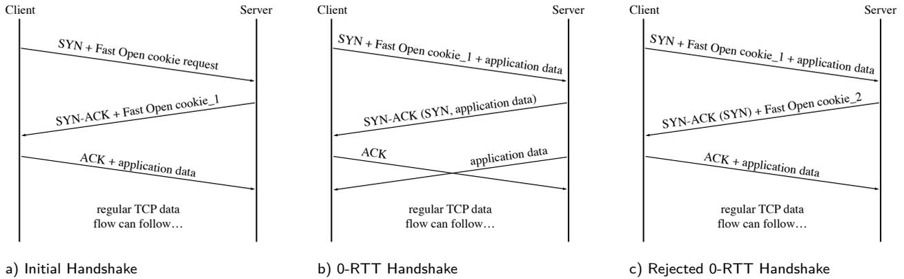
Fig. 1. Handshakes in TCP Fast Open protocol.
