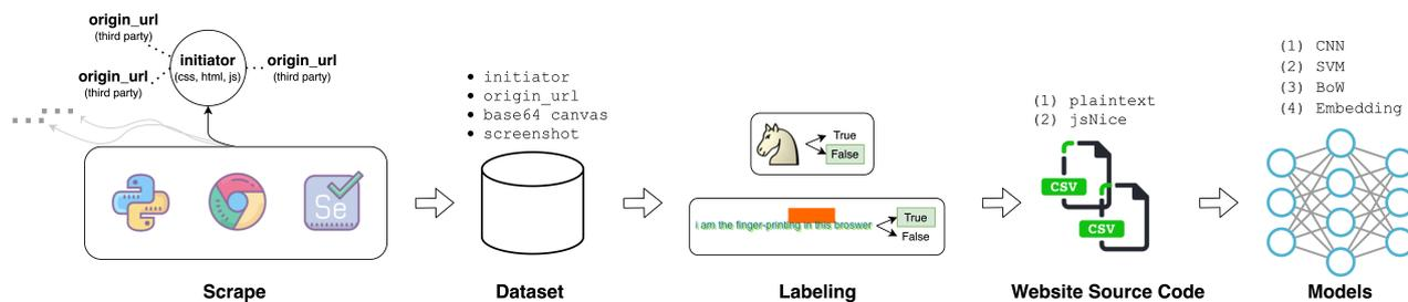
**Fig. 1.** ML-CB. We **scrape** (3.1) the web with a custom Chrome extension, adding a hook on the `toDataURL` function. The hook updates the **database** (3.2), storing canvas-related information. Canvas images, along with supporting material, are visually inspected for **labeling** (3.3). **Website source code** (3.5) associated with the images are then fetched and stored in either plaintext or jsNiceified form. Machine learning **models** (3.6) are trained on both images and text.
