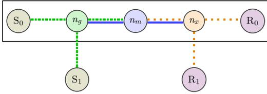
**Fig. 1.** Upper part: A Tor circuit consisting of a sender  $S_0$ , a guard node  $n_g$ , a middle node  $n_m$ , an exit node  $n_x$ , and a recipient  $R_0$ . Colored lines for each node depict the observations this node can make. Lower part: Further observations for an alternative sender  $S_1$  and for an alternative recipient  $R_1$  that will be used to define different anonymity notions.
