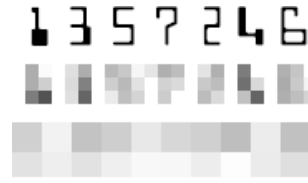
Fig. 5. Top row: a seven-digit string rendered in 24p MICR Encoding font. Middle and bottom rows: mosaiced images with grid sizes of 8p and 18p, respectively.
