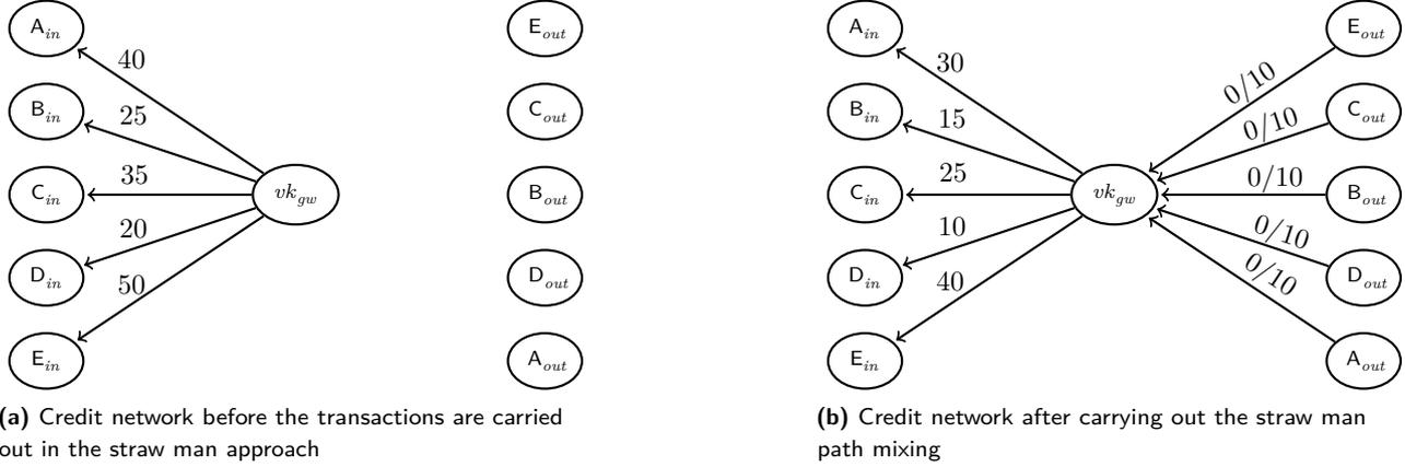
**Fig. 1.** An illustrative example of the straw man approach for path mixing to mix 10 IOU among five users. Solid arrows depict credit links between two wallets. Single values on edges denote the current balance and no upper limit. Values  $a/b$  on the links denote:  $a$  current balance and  $b$  upper limit. After finishing the straw man protocol, user A can perform a transaction for up to 10 IOU using  $A_{out}$  and  $vk_{gw}$  as the first hops in the transaction path.
