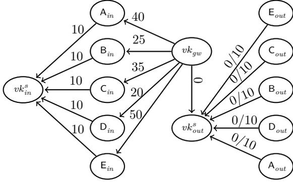
(a) Credit network after the set up of the shared wallets and output credit has been issued
