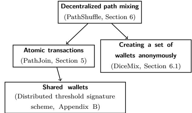
**Fig. 2.** Schema for a decentralized path mixing protocol. Boxes represent the functionalities denoted by the name in bold. Each functionality is implemented by the protocol in parentheses and it is described in the annotated section. An arrow  $a \rightarrow b$  denotes that protocol  $a$  depends on  $b$ .
