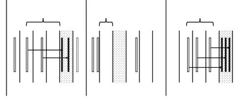
**Fig. 3.** To ensure invisibility, TagIt fingerprinter only moves  $R_{move}$  fraction of packets into fingerprint slots.  $R_{move}$  depends on the rate of the flow being fingerprinted.
