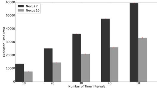
**Fig. 3.** Computational delay of cryptographic operations during join protocol in android devices.
