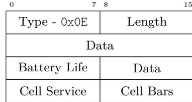
Fig. 5. Instant Hotspot Message - Frame Format
