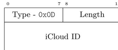
Fig. 3. Wi-Fi Settings Message - Frame Format
