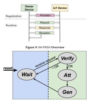
Figure 10: IM-PAISA State Machine on Idev
