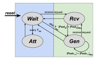
Figure 4: DB-PAISA State Machine on Idev
