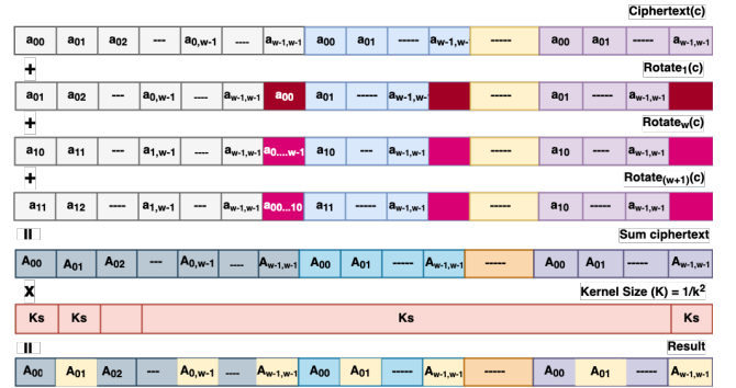
Figure 5: Secure Average Pooling with kernel size of k^2 . The resulting ciphertext is passed to a striding module.
