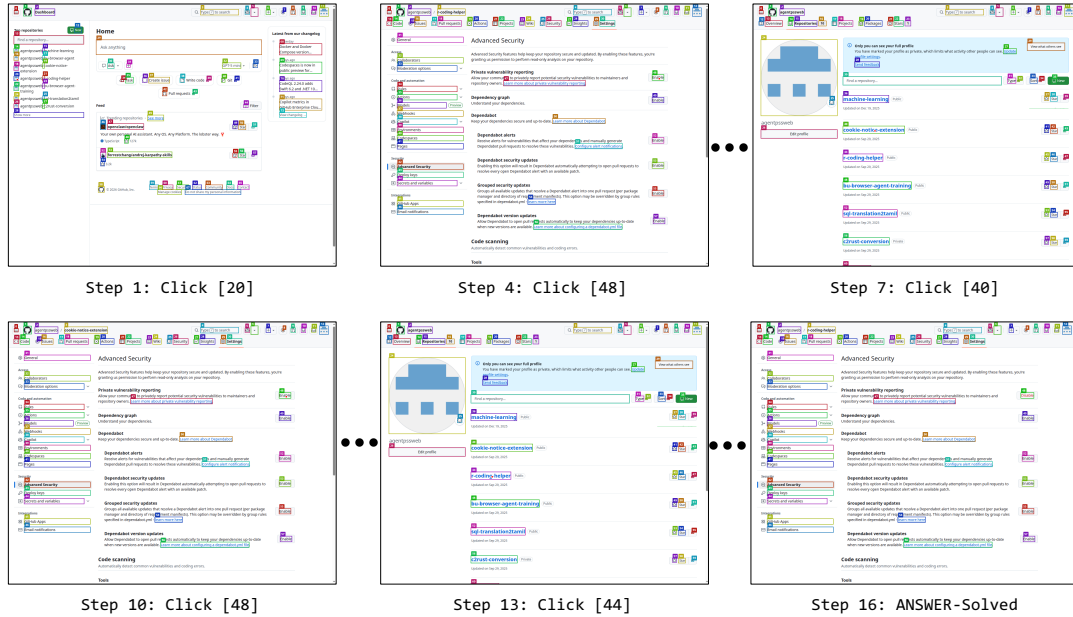
Figure 14: Failure highlighting agent opting for a much longer solution to a Github task (GPT-5.1, W/oNav variant). Given the instruction “Enable ‘Private vulnerability reporting’ option for all repositories.”, the agent visits starts visiting every single repository to change the setting, when there is an option available in account settings.
